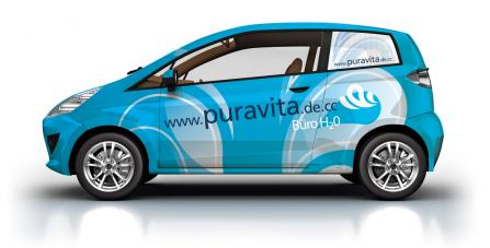
Cast 7-year film with SmartApply for demanding wrappings, e.g. over crimps and rivets in vehicles and other complex shapes
